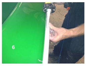
7. Continue around the aft corner, apply masking tape to keep it in place, half way along the side apply tape, around the bow, continue on back to stern. Expect to use about 2/3rds of a cartridge for a 303W.
